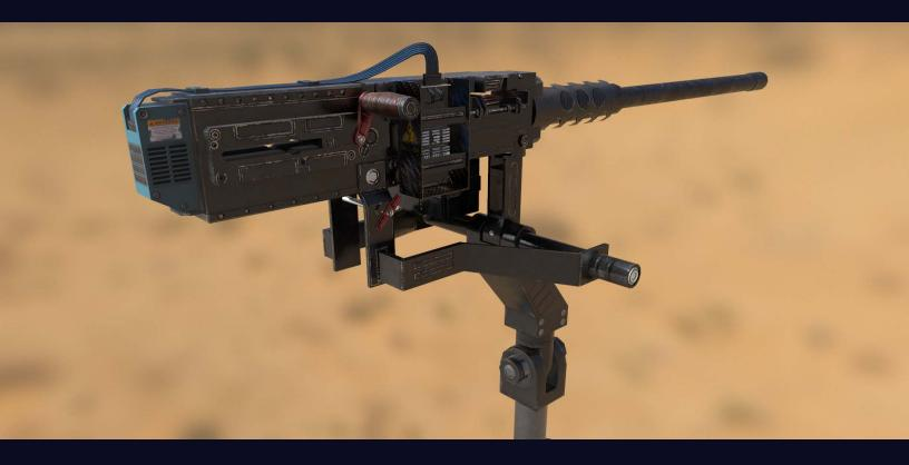
The M2c Browning is a computer-controlled version of an automatic, recoil operated, air-cooled machine gun with disintegrating metallic link-belt that is used to feed the ammunition into the weapon. Traditional spade grips and trigger were replaced with a digital trigger that is controlled by a small, single-board computer.
